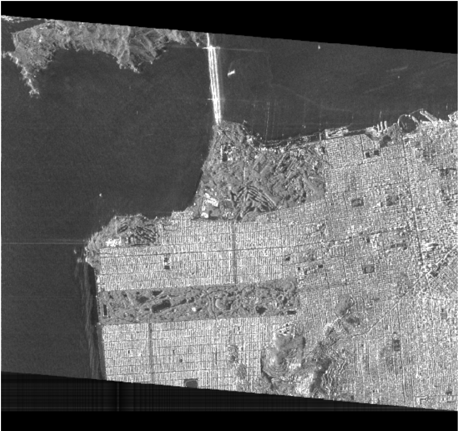
Fig. 2-25. Image of San Francisco, California, synthesized using a 45-deg linearly polarized antenna to transmit the signals and a 135-deg linearly polarized antenna to receive. Notice the increased contrast between the urban areas and the vegetated Golden Gate Park, as well as the contrast between the urban areas and the ocean.
