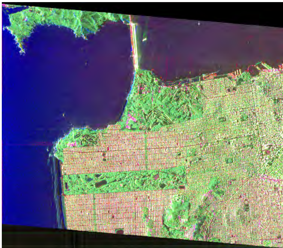
Fig. 3-9. Color overlay of San Francisco displaying |S_{hh} + S_{vv}| in blue, |S_{hh} - S_{vv}| in red, and |S_{hv}| in green. These three colors are the magnitudes of the scattering matrix elements when they are expressed in the Pauli basis.
