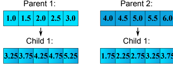
Figure 4.4 Illustration of the arithmetic crossover operator with \alpha = 0.25 .
