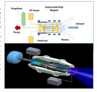
Fig. 3 VASIMR simplified diagram and cutaway.
