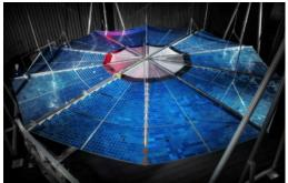
Fig. 4 20 kW MegaFlex testing at NASA GRC Plumbrook facility.
