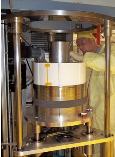
Fig. 4 Beryllium oxide radial reflectors (white) installed around centering ring and on Comet platen
