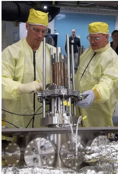
Fig. 2 Installing interference band clamps around HEU core and heat pipes inside DAF test area
