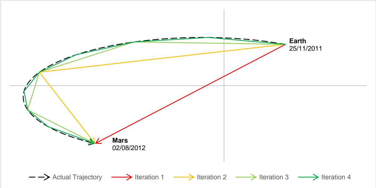
Figure 4.12 – Example of the first four iterations in the determination of the trajectory points of the Mars Science Laboratory mission.
