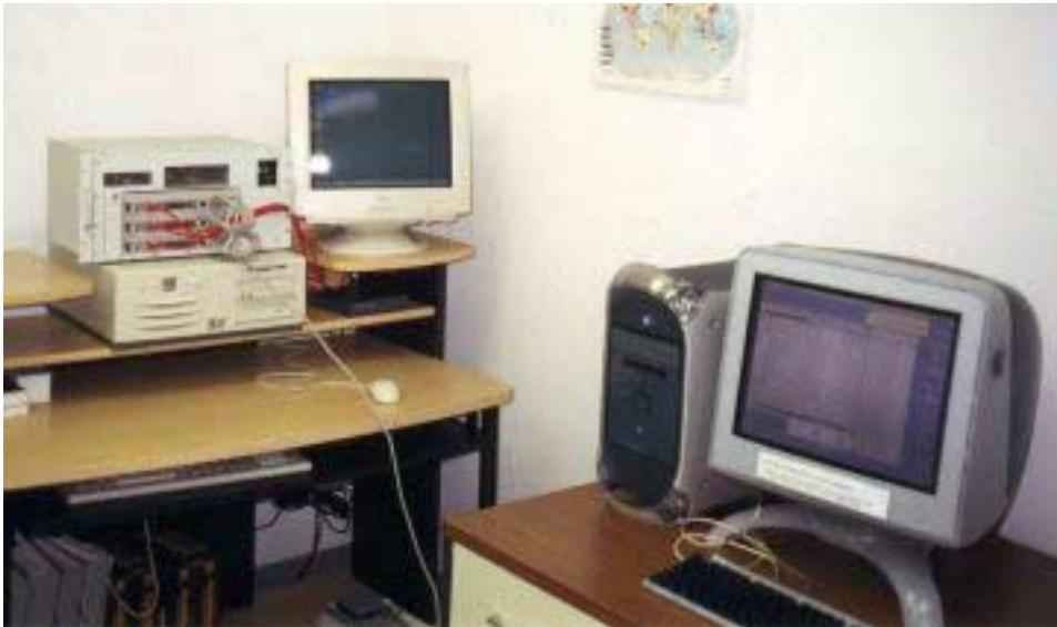
The multi spacecraft simulation, written in C++, runs on the Apple G4 machine. Three spacecraft are simulated and each has a separate Force 6750 board in the chassis on the left. The Dell machine is used for software development and hosts all of the developer tools. The simulation communicates with the boards using TCP/IP.
